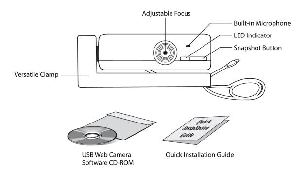
**▼ Note**: 1. The power supply for the camera is provided through the USB cable.
